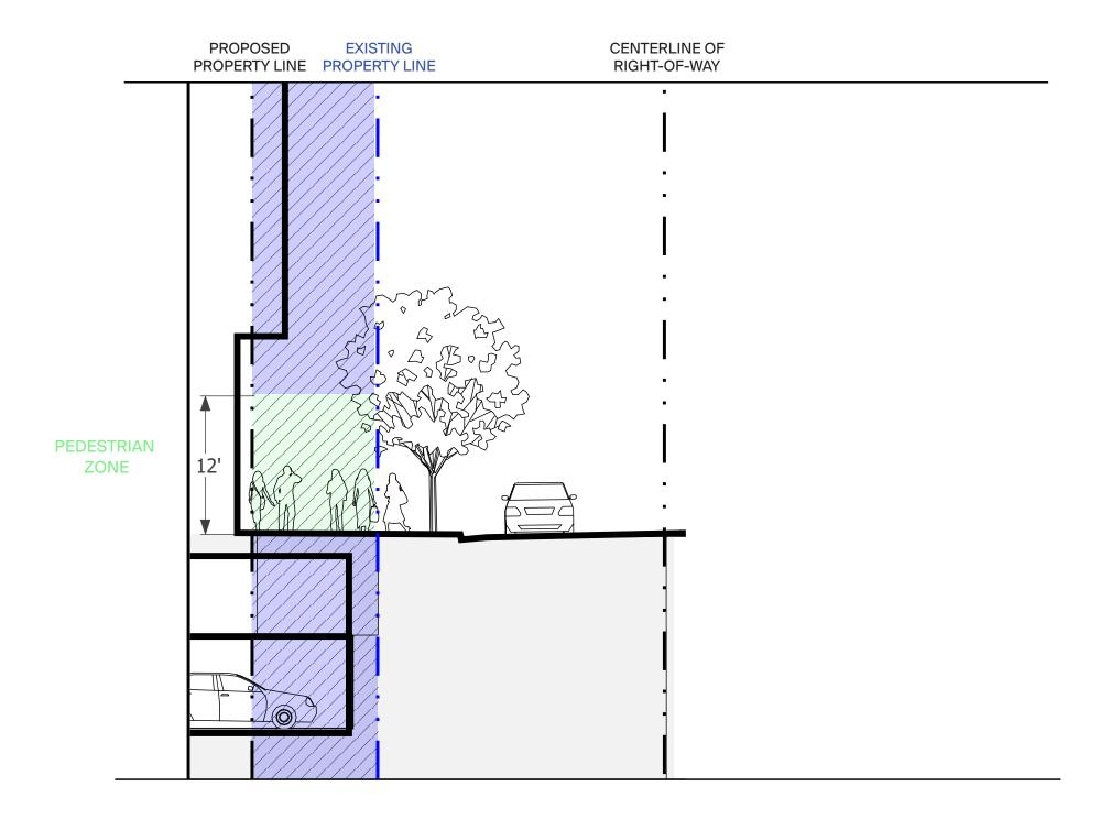
**Encroachment** As illustrated in Figure 10, structures may cantilever over or be built under right-of-way that is dedicated in this SP. However, a clear zone of 12' in height must be provided above sidewalks. Configuration subject to approval of Mandatory Referral and Fire Marshal access requirements
