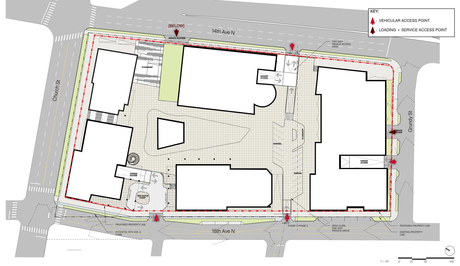
FIGURE 05 I VEHICULAR ACCESS DIAGRAM
